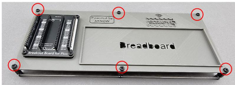
Step 5: Pill off the protective tape underneath the 830 pcs breadboard and place it on the “Breadboard” section of the Kit. Please make sure, the positive (+) side of the breadboard is on top as the following image indicates.
