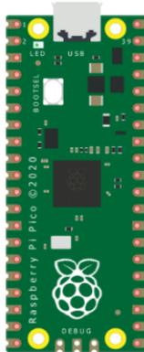
Plug the micro-USB cable into the port on the left-hand side of the board.
