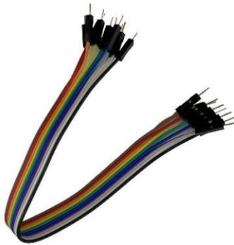
Jumper cables/ wires are simply wires that have connector pins at each end, allowing them to be used to connect two points to each other without soldering. Jumper wires are typically used with breadboards and other prototyping tools in order to make it easy to change a circuit as needed. The colour variation of the wires can be used as advantage in order to differentiate between types of connections, such as ground or power.
